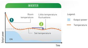
NOTE: Saves energy by varying the rotation speed of the compressor to maintain the set temperature.
