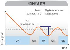
NOTE: Energy is wasted by switching the compressor ON and OFF to maintain the set temperature.
